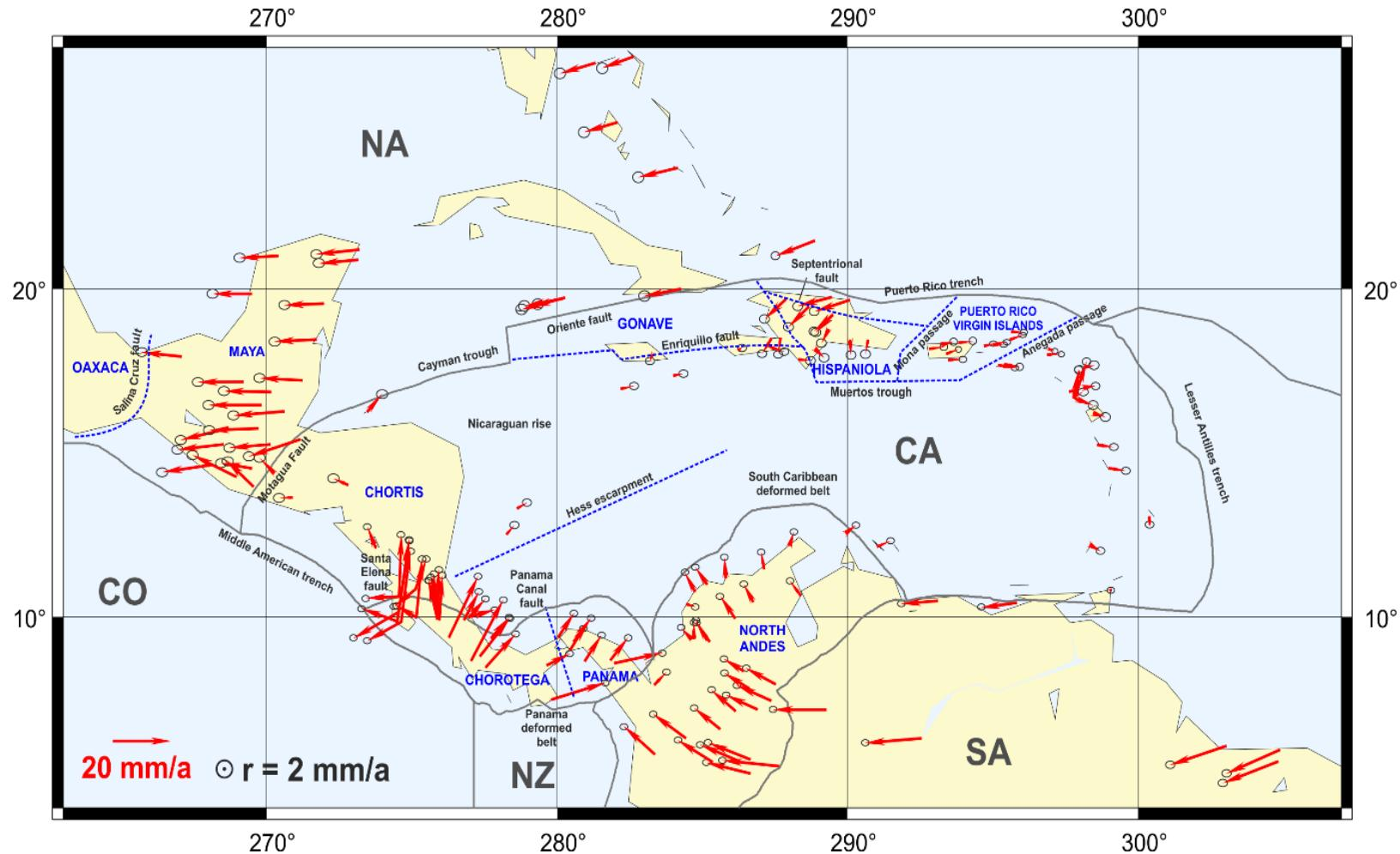
Geodetic station velocities relative to the Caribbean plate and block geometry used for the computation of the deformation model. Plate boundaries (in black) after Bird (2003), additional main tectonic blocks (in blue) after Boschmann et al. (2014), James (2007), Symithe et al. (2015) and Calais et al. (2016). CA: Caribbean, CO: Cocos, NA: North America, NZ: Nazca, SA: South America.
