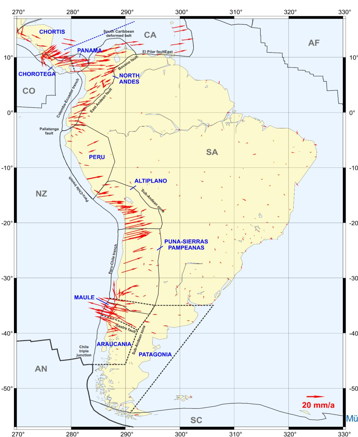
Geodetic station velocities relative to the South American plate and block geometry used for the computation of the deformation model. Plate boundaries (solid black lines) after Bird (2003), additional tectonic blocks (dashed lines) inferred from the station velocity behaviour. Plates: AF: Africa, AN: Antarctica, CA: Caribbean, CO: Cocos, NZ: Nazca, SA: South America, SC: Scotia..
