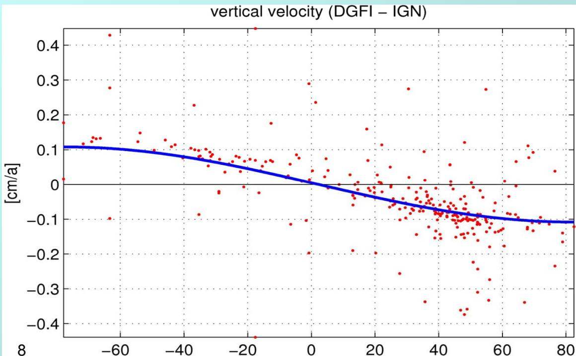
The good fit of the sine of latitude function indicates a translation of the network in z-direction
