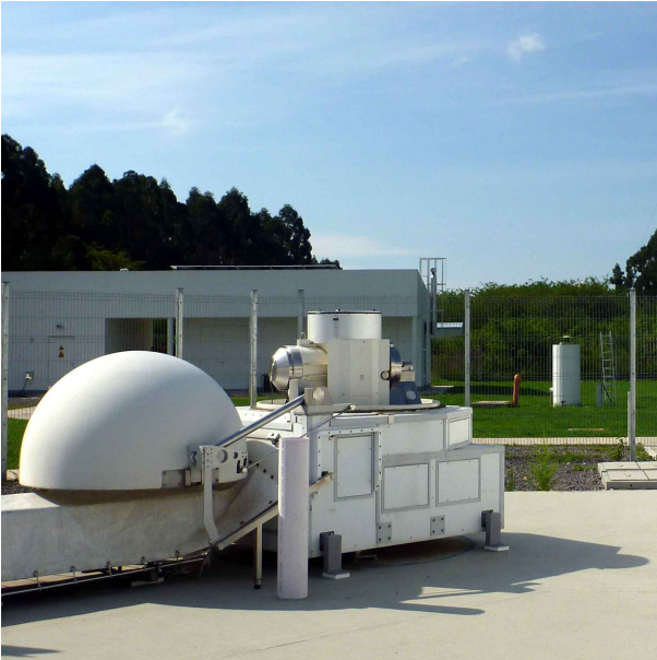
optical telescope with 50cm aperture laser system to measure distances
