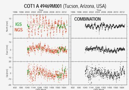
Figure 5: Residual position time series with respect to cumulative solution of individual weekly regional solutions (left) and weekly combined solution (right).
