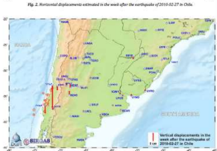
Fig. 3. Vertical displacements estimated in the week after the earthquake of 2010-02-27 in Chile.
