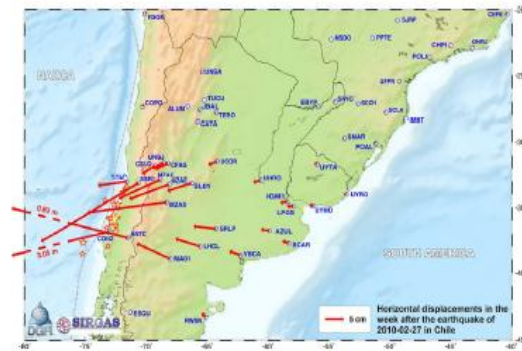
Fig. 2. Horizontal displacements estimated in the week after the earthquake of 2010-02-27 in Chile.
