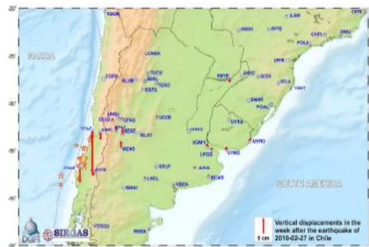
Fig. 3. Vertical displacements estimated in the week after the earthquake of 2010-02-27 in Chile.
