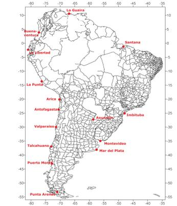
Fig. 8. Reference tide gauges and vertical networks of the existing height systems in South America.
