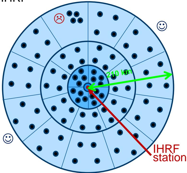
**Template according to the gravity effect on the geoid**
