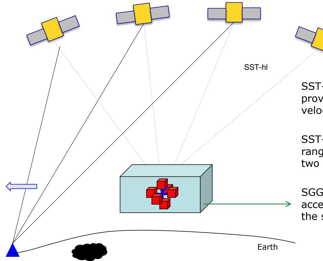
SST-hl: The high-orbiting satellites (e.g. GPS) provide highly accurate 3D position information, velocity and acceleration of the LEO
