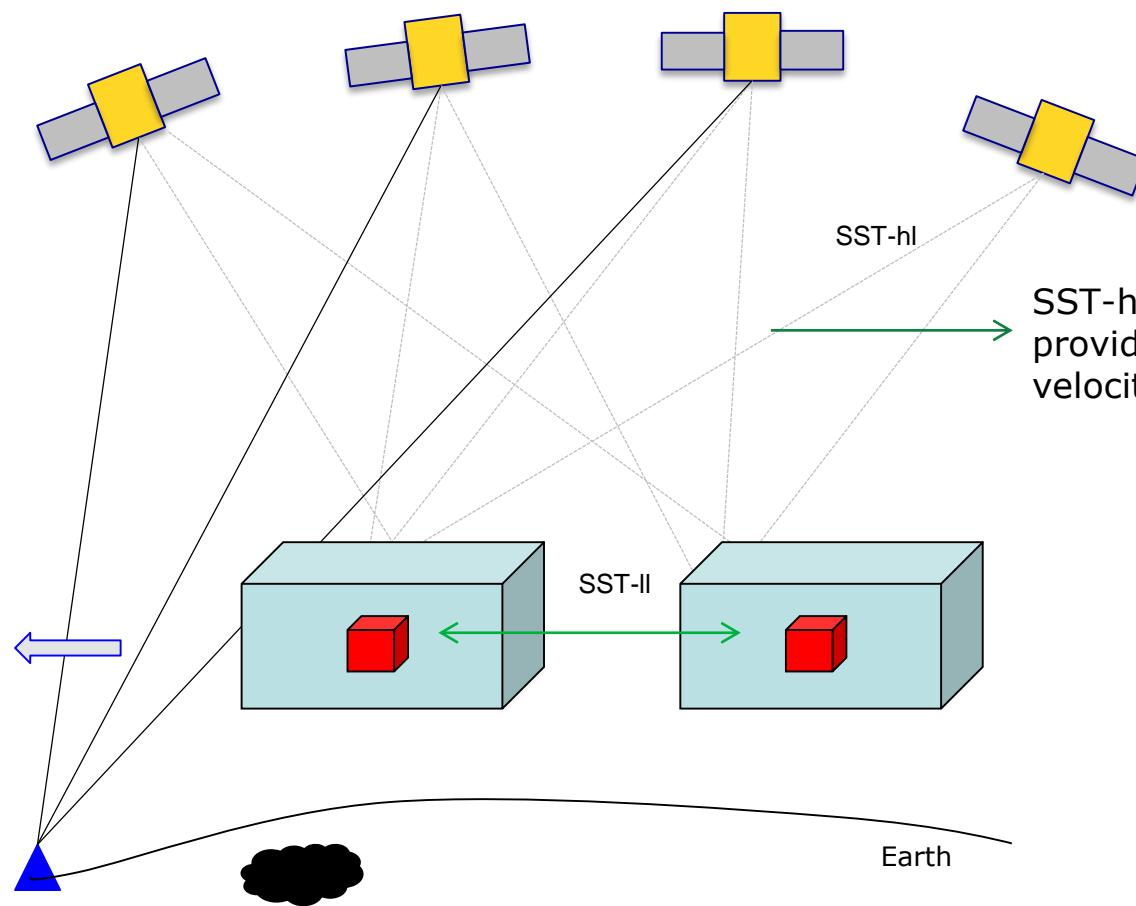
SST-hl: The high-orbiting satellites (e.g. GPS) provide highly accurate 3D position information, velocity and acceleration of the LEO
