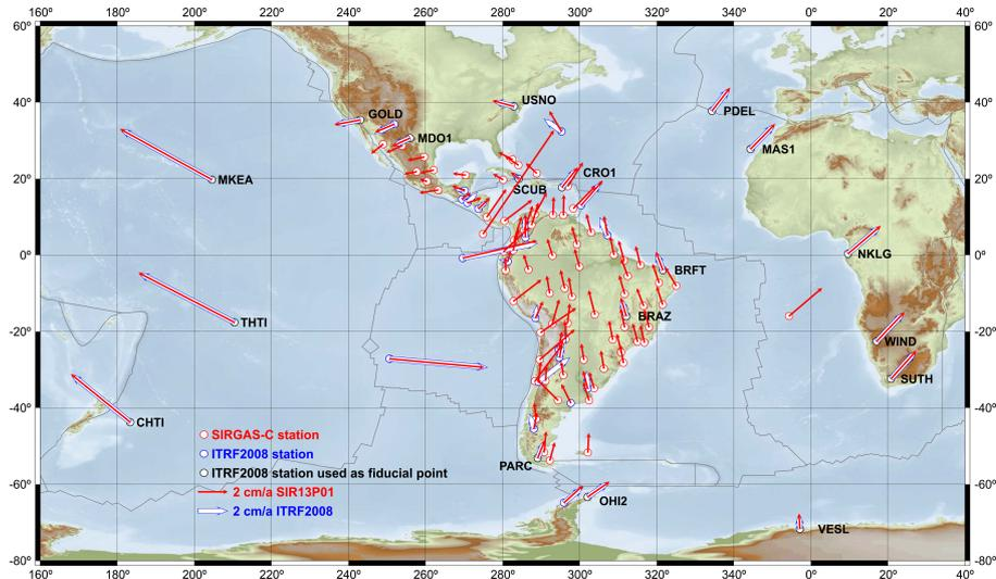
**Figure 2:** Horizontal velocities of the SIRGAS multi-year solution SIR13P01: it covers the time span from April 2010 to June 2013, includes 108 SIRGAS core stations and refers to ITRF2008, epoch 2012.0. (Stations with labels are fiducial points).
