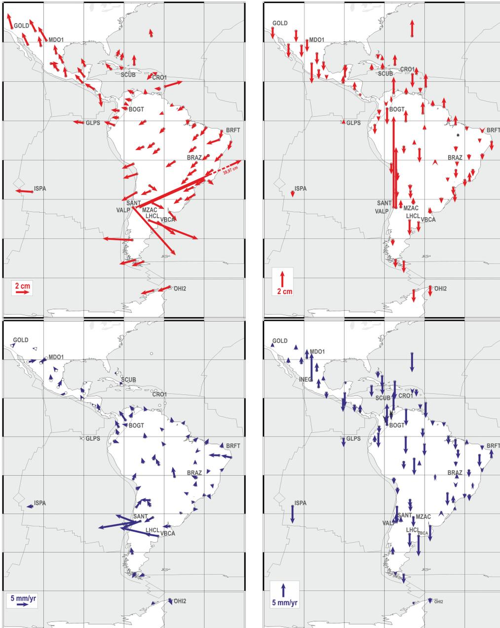
**Figure 4:** Horizontal (left) and vertical (right) residual position (upper two figures) and velocity (lower two figures) vectors between the SIR10P01 (before the earthquake in February 2010) and the SIR13P01 solutions.
