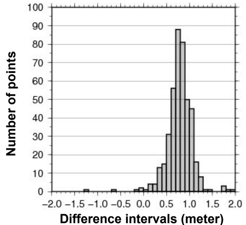
Histogram of differences of geodetic heights of GPS points over Bench Marks with those obtained by GEOSULv2
