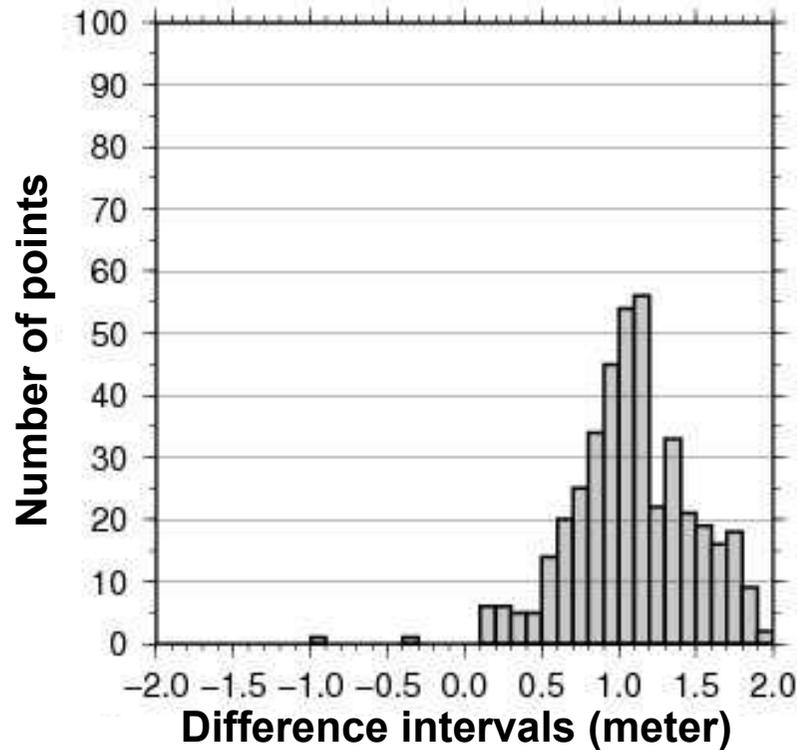
Histogram of differences of geodetic heights of GPS points over Bench Marks with those obtained by GEOSULv1
