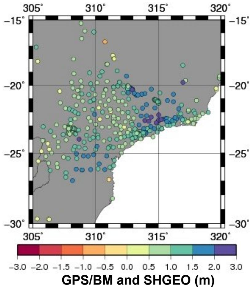
Comparison with the geodetic heights obtained by GEOSULv2.
