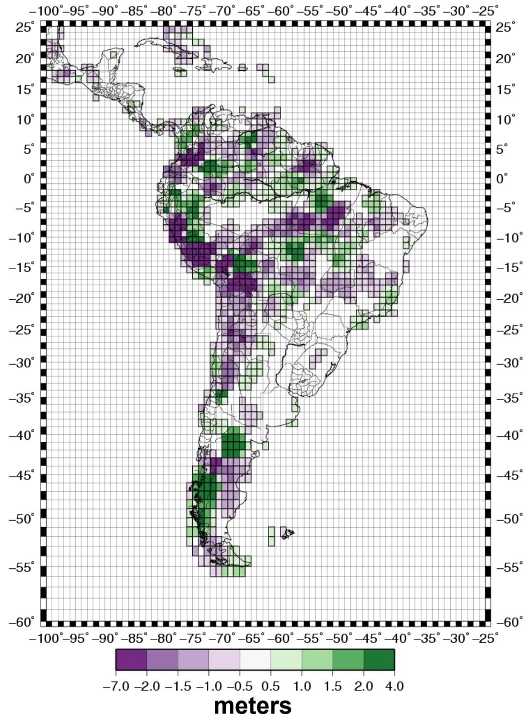
Differences between GPS geoidal heights in 995 points on BMs and height anomalies from EGM96, EIGEN-GL04C and PGM2007A (n=m=360)
