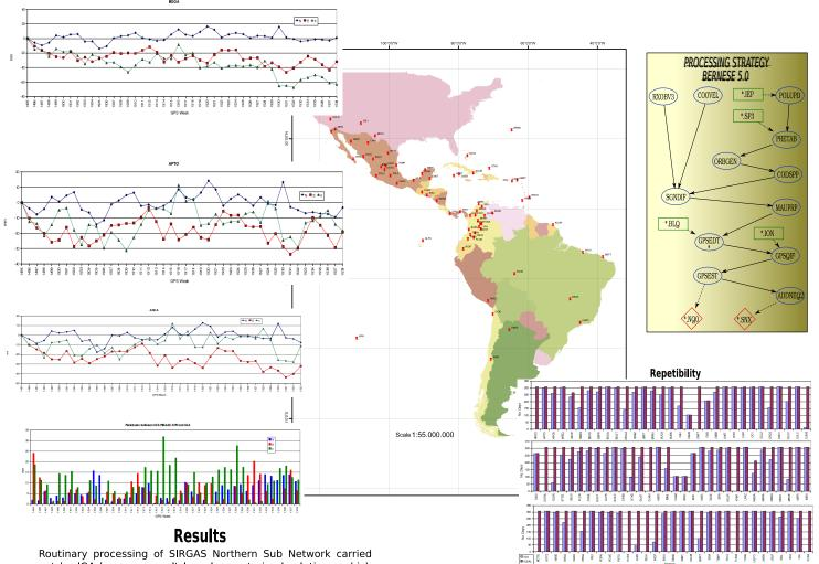
Routinary processing of SIRGAS Northern Sub Network carried out by IGA has as a result loosely constrained solutions, which are upload to disposition of Combination Centers through DGFI's FTP into daily normal equations and one weekly SINEX file. These SINEX contains all statistical information necessary to rebuild corresponding normal equation
