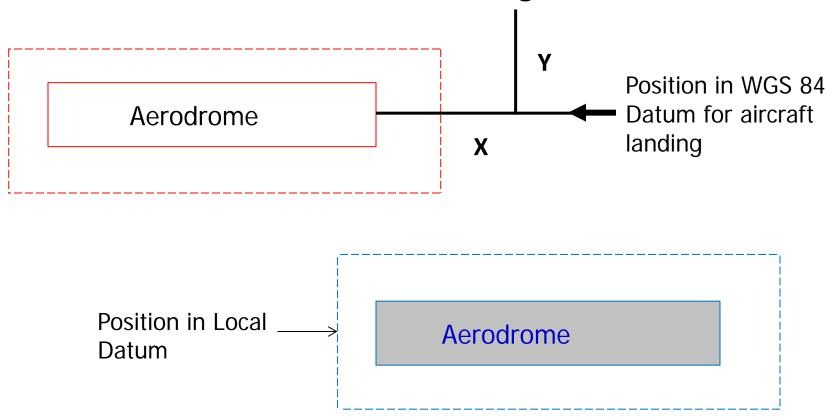
ICAO goal - To make Local Datum aligned to WGS 84 making Air Navigation safer
