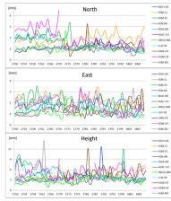
Time series of the RMS of the station position residuals for each analysis centre with respect to the IGS weekly solutions. This comparison allows to assess the accuracy of the individual solutions; i.e. about  $\pm 2$  mm in the North and the East, and  $\pm 5$  mm in the height.
