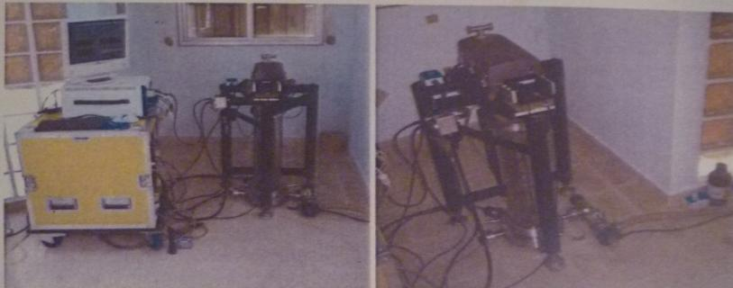
Figure 4.8.3. Pictures of the IMGC-02 at the observation station in Panama City - IGNTG - CORS
