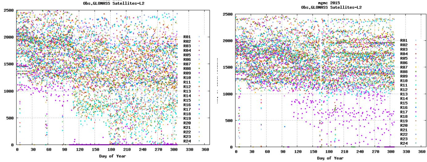
Stations MCL1 and MGMC are less than 1 km far from each other but MCL1 has wrong configuration as can be seen in the plots of GPS observations L1 and L2 of both stations. MCL1 is not collecting block. In All stations can be seen a different behavior of GLONASS after day 180 of 2015
