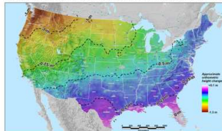
Predicted change estimated as NAVD88 "zero" (datum) surface minus NGS gravimetric geoid
