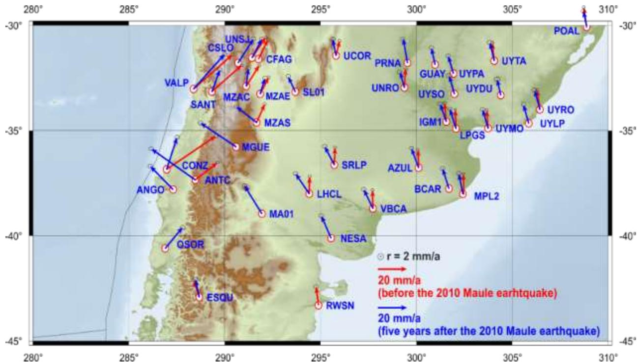
Station velocities determined before and five years after the 2010 Maule earthquake. Velocities were oriented about N45°E before and N40°W after the event (~20 mm/a).
