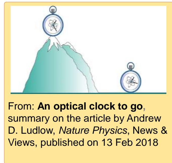
Excellent agreement between height differences from clock and from conventional geodesy: 0.19 m, but clock accuracy still two orders of magnitude below geodesy
