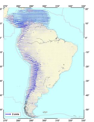
Fig. 6. Surface deformation models relative to the South American plate: VEMOS2009 (left) valid from 2000.0 to 2009.6; VEMOS2015 (centre) valid from 2012.2 to 2015.2; VEMOS2017 (right) valid from 2014.0 to 2017.1.
