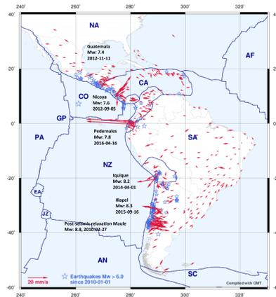
Fig. 4. Changes in the velocities of the SIRGAS stations caused by strong earthquakes since February 2010.
