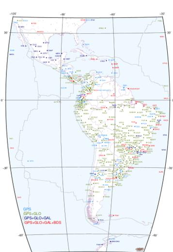
Fig. 3. Present SIRGAS reference frame: it comprises 533 continuously operating GNSS stations: 67 belonging to the IGS global network, 339 tracking GLONASS, 79 tracking GALILEO, and 43 tracking BEIDOU. 122 stations have been decommissioned, but they are included in the SIRGAS reprocessing campaigns.
