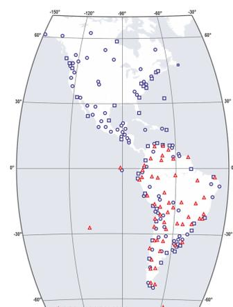
Fig. 2. SIRGAS reference frames SIRGAS95 and SIRGAS2000 (based on GPS campaigns in 1995 and 2000, respectively).
