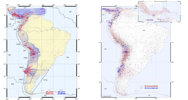
Fig. 6. Surface deformation models relative to the South American plate: VEMOS2009 (left) valid from 2000.0 to 2009.6; VEMOS2015 (centre) valid from 2012.2 to 2015.2; VEMOS2017 (right) valid from 2014.0 to 2017.1.
