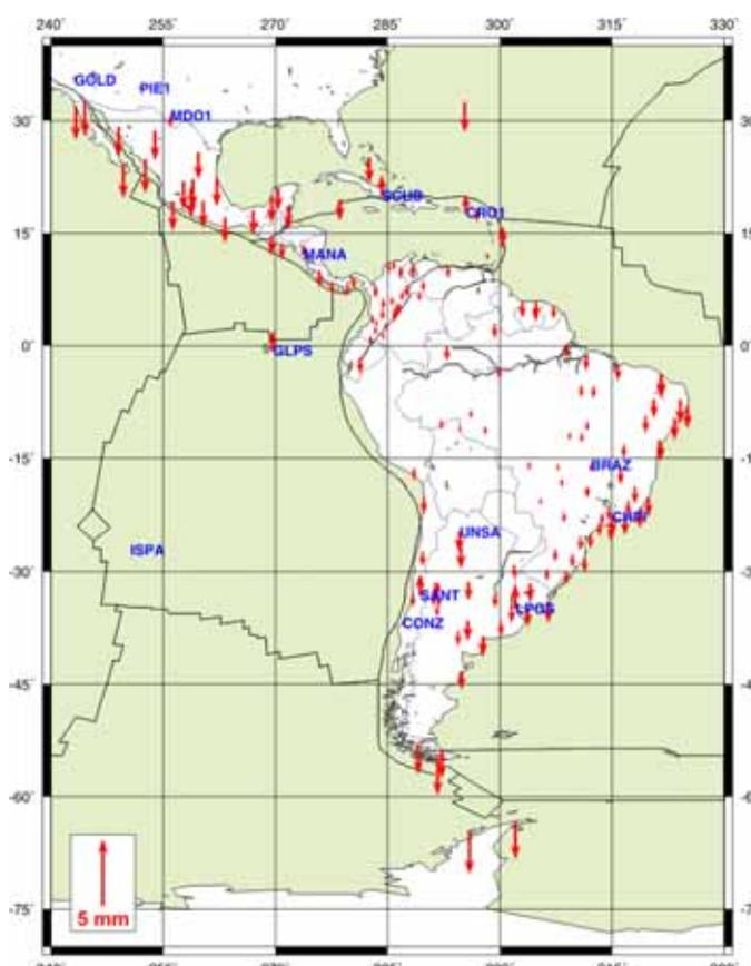
Discrepancies wrt loosely constrained solutions after applying different reference coordinates for the datum definition (GPS week 1504)
